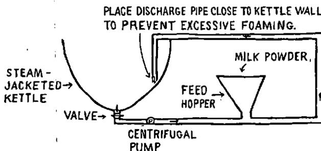
solved is merely dumped into the hopper and the action of the water passing through the pipe continuously draws in small amounts of powder, resulting in rapid and thorough mixing of powder and liquid.
